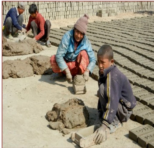
Workers making bricks
